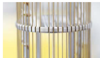
▲ ICE can offer customised experimental wiring including up to 100 coax lines on systems in the DRY ICE 1K Series
